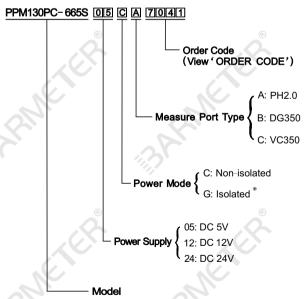
When choose isolated power mode, signal's unbalanced input cannot
